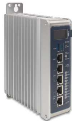
Figure 2: Industrial controllers capable of virtualization, such as Emerson’s Outcome Optimizing Controller (OOC), include multiple processing cores, digital communication ports, and support for parallel operation of a control RTOS and a general-purpose OS.
